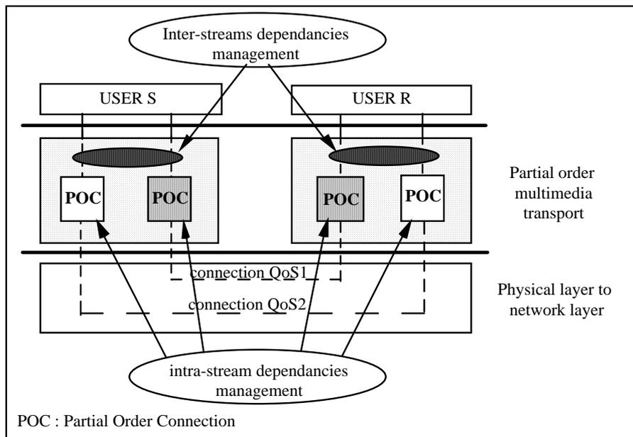
**Figure 5.** Architecture of the sending and receiving entities of a partial order transport
