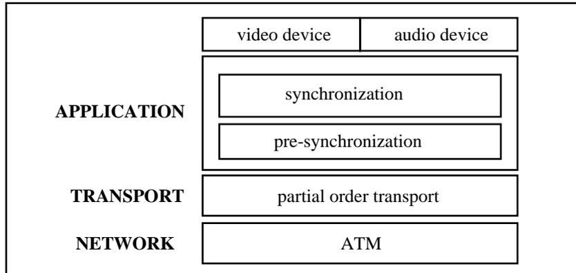
**Figure 9.** *PNSVS architecture on top of a partial order transport service*
