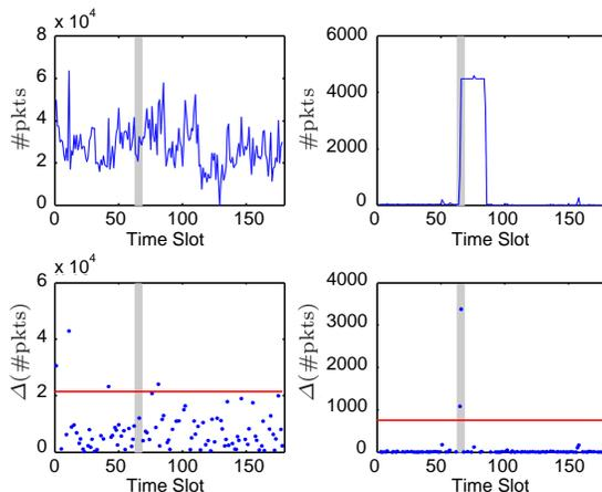
**Fig. 2.** Low-intensity anomalies might be hidden inside highly aggregated traffic, but are visible at finer-grained aggregations. The DDoS attack is evident at the victim’s network.
