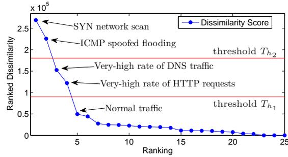
(a) Detecting network attacks using dissimilarity vector  $D$ .
