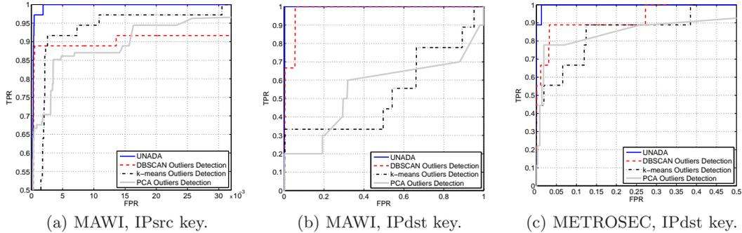
**Fig. 5.** True Positives Rate vs False Alarms in MAWI and METROSEC.
