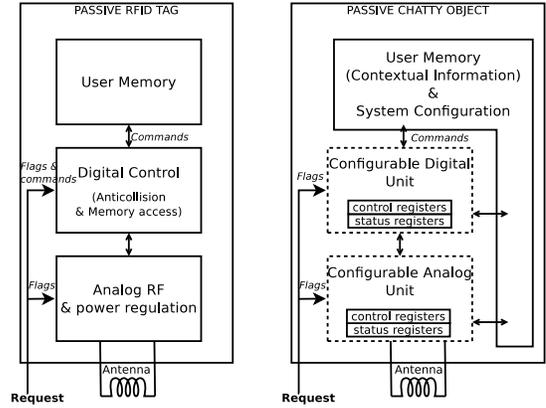
Fig. 2: Here are two simplified diagram block. On the left is a common RFID tag design. Its communication is driven by the flags field of the request and by others few specific commands. On the right, the behavior of a chatty object is configurable from the reader by accessing internal register or configuring programmable units.
