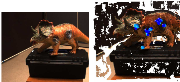
Fig. 5. Left : The left eye’s image of figure 4’s scenery. Right : The pose of the object is successfully determined using Rigid Motion minimization.
