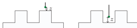
FIG. 4. Definition of z near the rough bottom plate, above a plot, or inside a notch.
