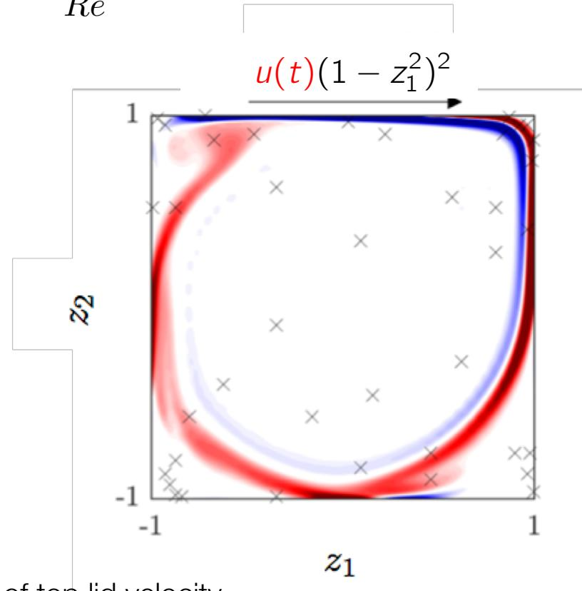
**Control input:** Amplitude of top lid velocity
