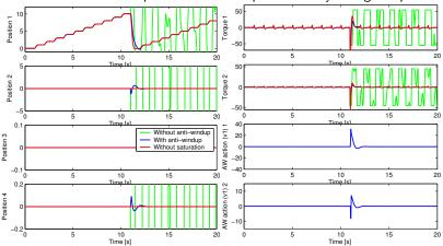
The anti-windup action dies away to recover the unconstrained closed-loop
