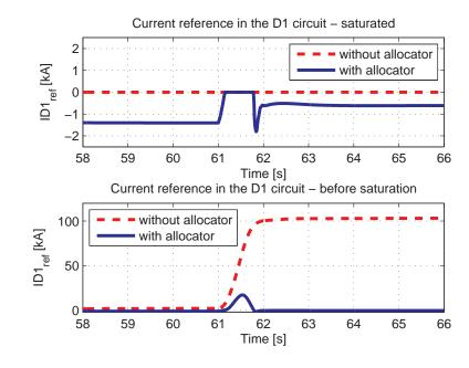
With the allocator, current in the D1 circuit saturates only during the transient (upper figure, blue).
