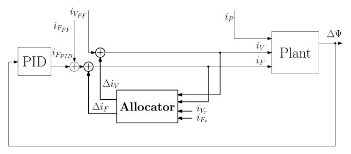
ightharpoonup Zoom of the allocator block (note the drift term  $u_0=u_r$  which is now a reference signal for  $I_F$ )
