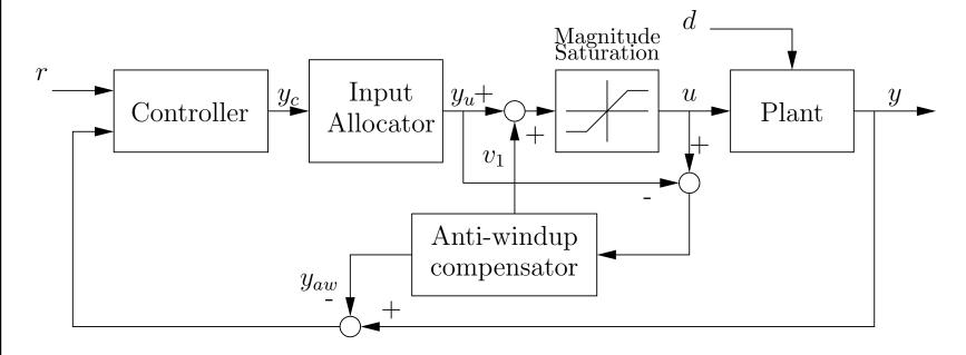
▶ Interpretation: anti-windup deals with saturation during transients; dynamic allocation avoids saturation at the steady-state
