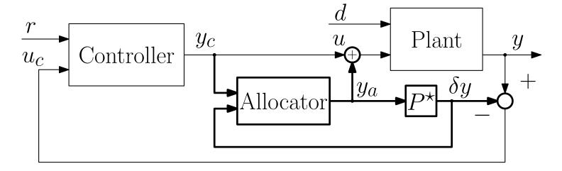
$\triangleright$  The signal  $P^*y_a$  ensures that the allocator does not "fight" against the controller at the steady-state (use two time scales again in proof)
