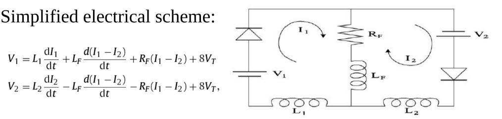
When incorporating the diodes in the equations (nonlinear):
