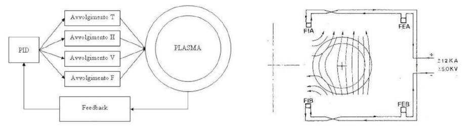
• The coil is controlled in feedback by a PID controller driving a circulating current 4 quadrants current amplifier
