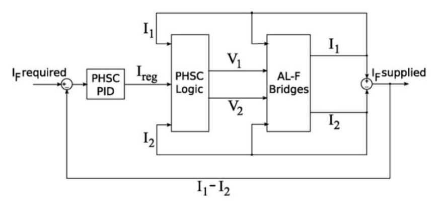
• PHSC Logic is a nonlinear block ensuring that the bridges provide currents *I1*, *I2* both above the lower conduction limits of the thyristors (1200 A)
