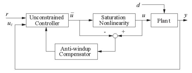
Dynamic allocation: address steady-state input specs
