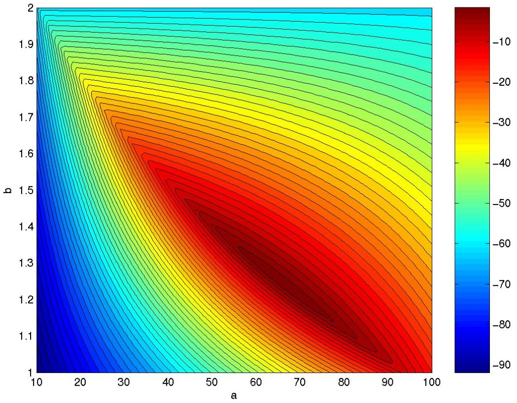
Figure 6: Value of  $\min_k g_x(a, b, d)$  as a function of  $a$  and  $b$  when  $d = 10.0938$  for the simultaneous stabilization problem given by Problem II. Simultaneous stabilization is ensured only for positive values (in dark red).
