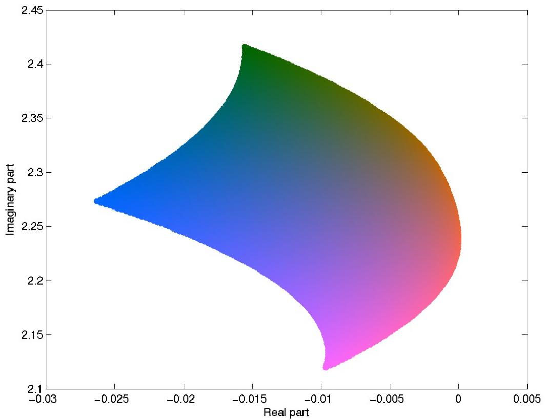
Figure 5: Robust root locus of the dominant pole for the robust stability analysis of Problem I. The dominant pole remains on the left hand side of the complex plane.
