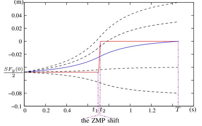
Fig. 2. We consider the upward half-step of Fig. 1, and show in red the corresponding  $p_y(t)$ . To this trajectory correspond an infinity of  $C^2$  solutions for  $y(t)$  which all verify  $y(0) = p_y(0) = \frac{SF_y(0)}{2}$ , each of them being fully defined by  $\dot{y}(0)$ . We show several such  $C^2$  solutions; the curve in blue is the solution retained: it is the unique one verifying  $y(T) = 0$ .
