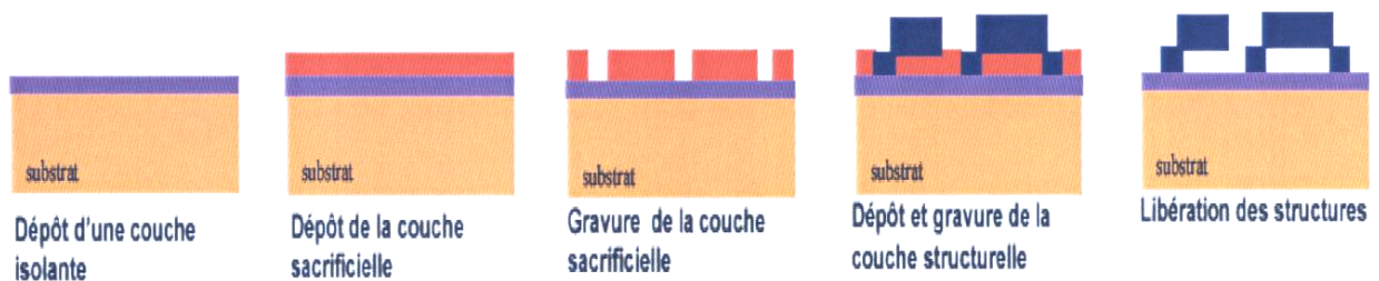
Figure 20: Principe du micro-usinage en surface
