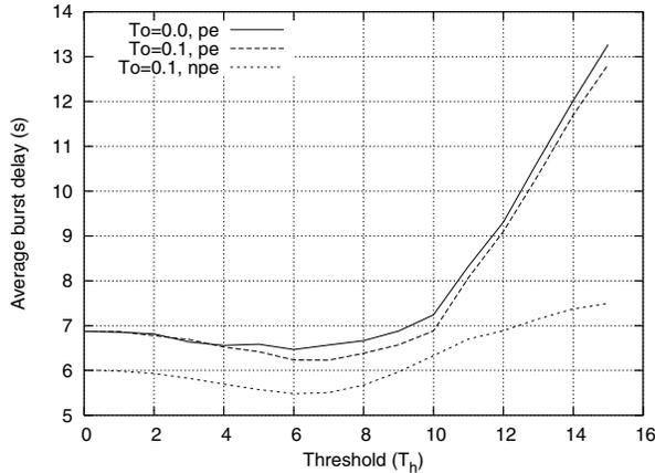
Fig. 7. Average Delay vs.  $T_h$ .  $N_{dch} = 1, N_{tcp} = 5, D_w = 500ms$ .
