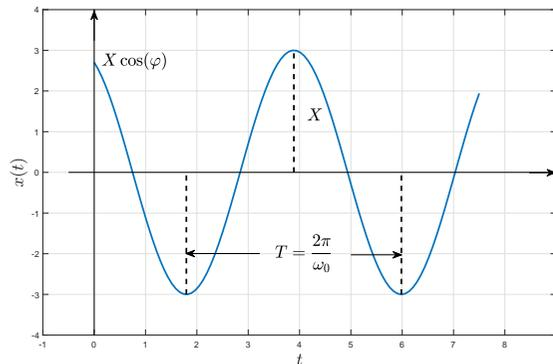
$$x_h(t) = \frac{v_0}{\omega_n} \sin(\omega_n t) + x_0 \cos(\omega_n t) = X \cos(\omega_n t + \varphi)$$
