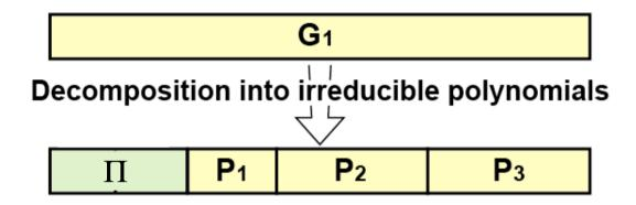
■  $\Pi$  = small degree polynomial featuring "standard" error detection properties (e.g., [1+x] => detection of odd-weight errors)
