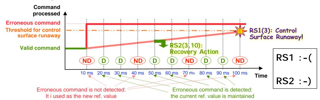
Target UE: Reception of 3 erroneous messages in a set of 10 cycles
