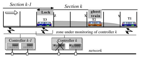
Fig. 2: Intersection handover with duplex controllers
