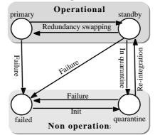
Fig. 5: Modes of operation of a fail safe unit
