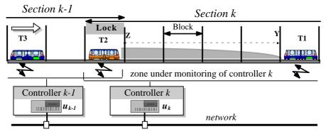
Fig. 1: Intersection handover with simplex controllers
