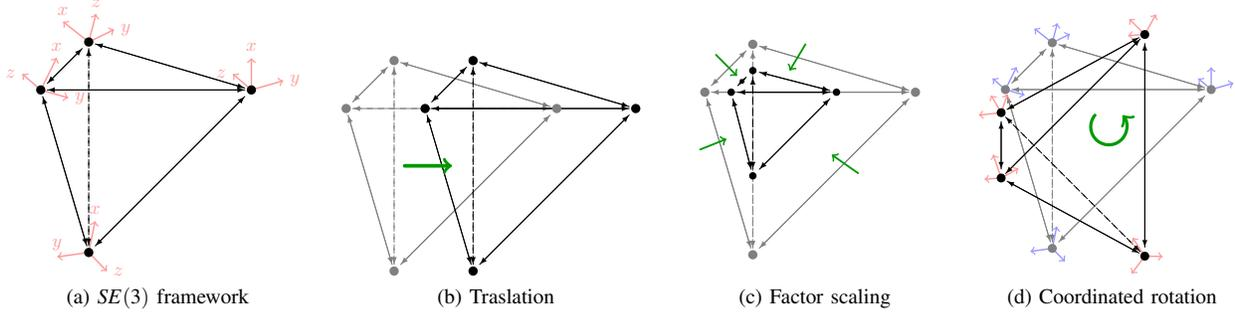
Fig. 2: Example of infinitesimal motions: the  $SE(3)$  framework  $(K_4, \mathbf{p}, \mathbf{a})$  (Fig. 2a) is translated along the  $x$  axis (Fig. 2b), scaled by a factor  $\alpha = 0.5$  (Fig. 2c), counterclockwise coordinated rotated of  $\theta = \pi/4$ rad (Fig. 2d).
