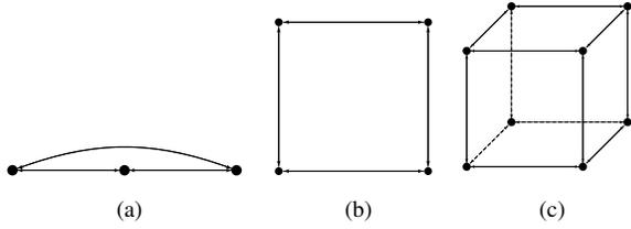
Fig. 3: Examples of non-infinitesimally  $SE(3)$ -rigid frameworks.
