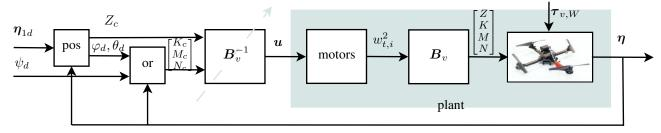
Fig. 2. Sketch of the control loop
