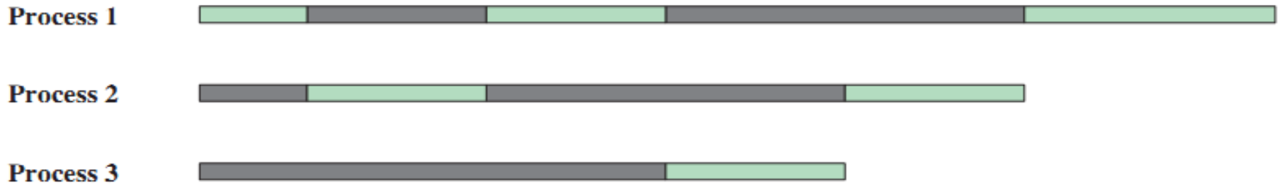
(a) Interleaving (multiprogramming, one processor)
