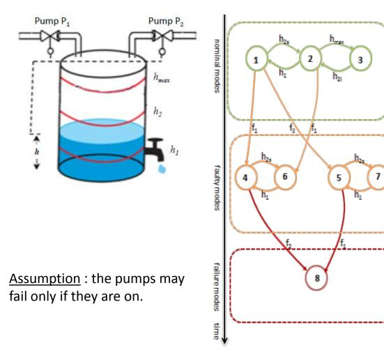
3 sensors: h<sub>1</sub>, h<sub>2</sub>, h<sub>max</sub> Pump control signals : ON, OFF
