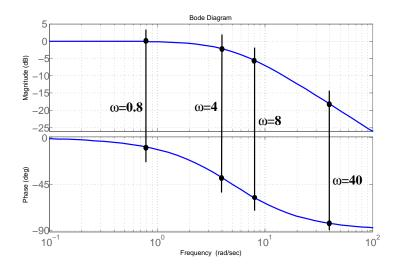
Frequency analysis consists in studying the response of a LTI system with sine inputs
