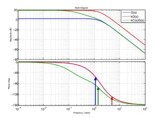
Phase margin: now, with the proportional gain and the phase lag controller  $=70^{\circ} \text{ (at } 1.56 \ rd/s)$
