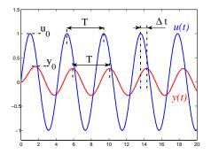
The output signal is also a sine with the same frequency, but with a different magnitude and a different phase angle.
