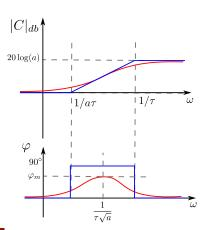
The phase lead compensator is used to increase the phase margin
