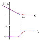
The phase lead controller is an approximation of the PD controller
