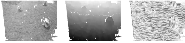
Figure 2: A result of our stereovision algorithm: from left to right, original image (only correlated pixels are shown), disparity image, and standard deviation on the disparity estimated with our error model.
