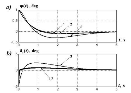
Yaw angle and rudder deflection for control  ${\bf K}_2$  and for  $h=0.1\ ,\ 5\ ,\ 9$
