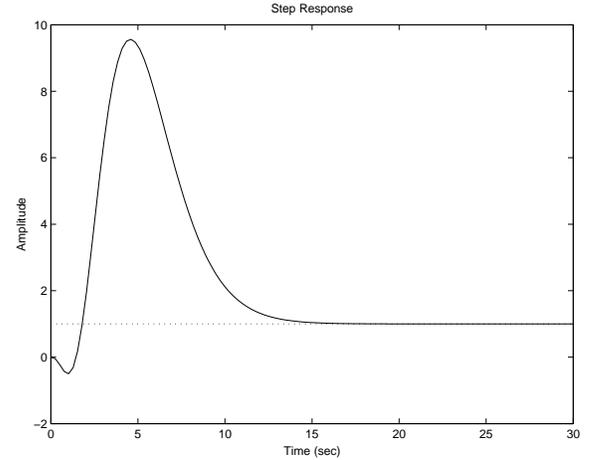
Fig. 2. Flexible mode controlled by initial controller. Closed-loop response to a step with unacceptable overshoot.
