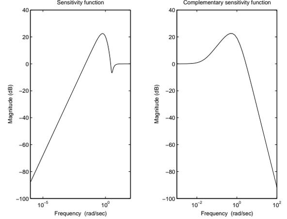
Fig. 1. Flexible mode controlled by initial controller. Closed-loop frequency-domain characteristics with large peaks.
