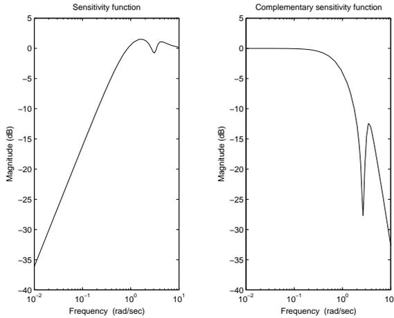
Fig. 3. Flexible mode controlled by optimized second-order controller. Closed-loop frequency-domain characteristics.
