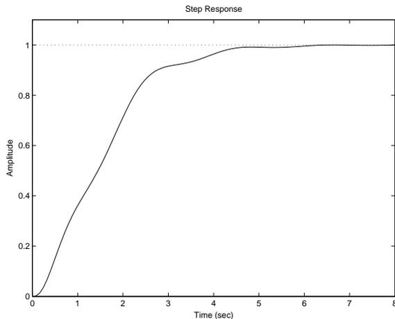
Fig. 4. Flexible mode controlled by optimized second-order controller. Closed-loop response to a step.
