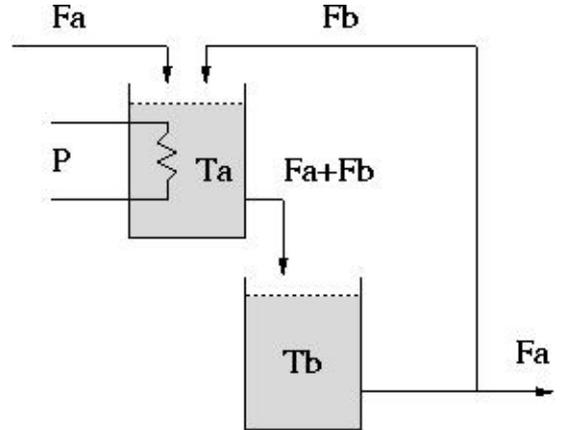
Figure 5: Two-tank system.
