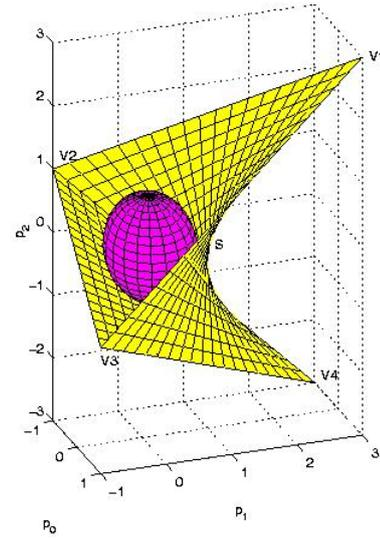
Figure 3: Hyperbolic and ellipsoidal stability domains for a third-degree discrete-time polynomial.
