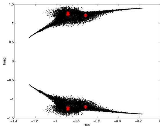
Figure 9: Robust root-locus of the wing.
