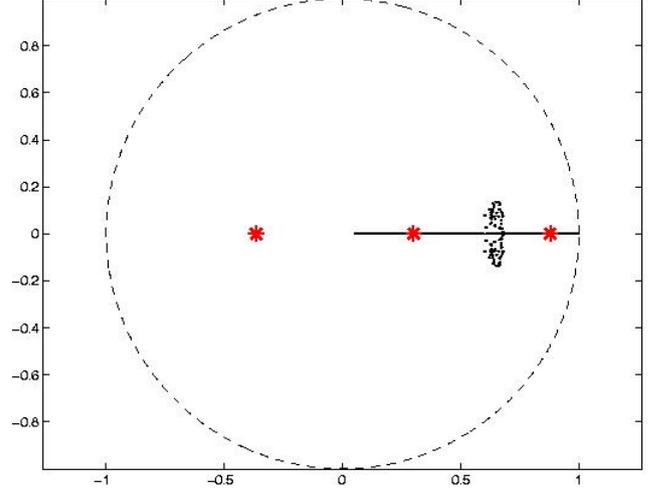
Figure 6: Root-locus within the unit disk.
