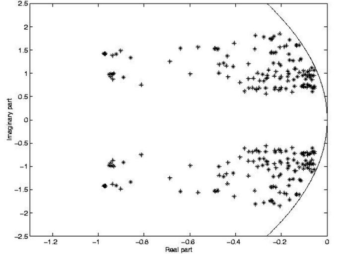
Figure 2: Roots of the 64 polynomial matrix vertices of the mechanical system.
