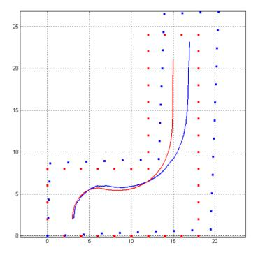
Figure 3. The planned trajectory in the map of the environment. Red dots reprensent the mean value of the stochastic map. The red line represents the trajectory planned based on this stochastic map. Blue dot represent a possible real position of the landmarks and the blue line represent the trajectory that would be actually followed by the robot in this environment by performing localisation on the landmarks.
