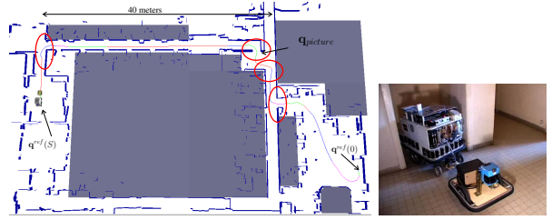
Fig. 9. On the left, the trace of collision free long-range navigation with robot Hilare2 towing a trailer. Red ellipses display locations where localization discontinuity may occur, because the visible landmarks change suddenly. Configuration \mathbf{q}_{picture} is visible on the right picture.
