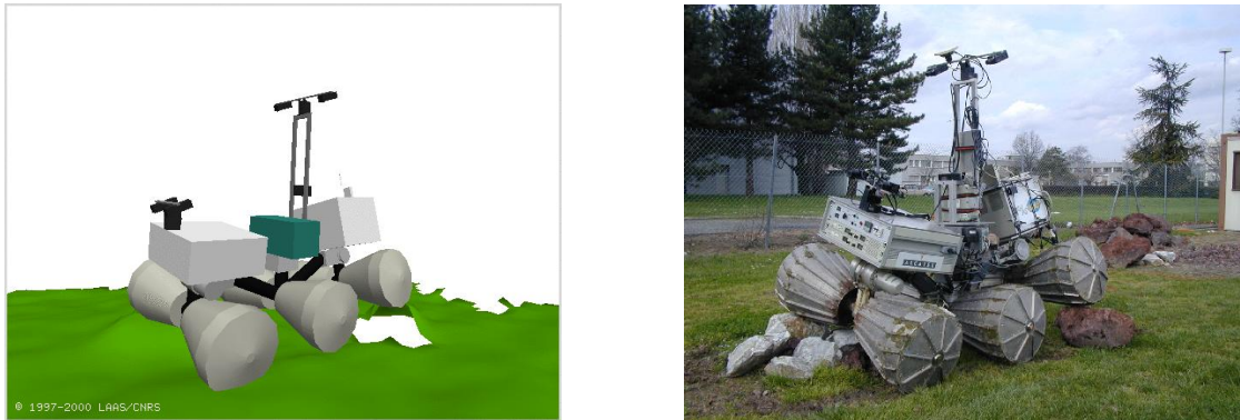
Fig. 7. A predicted placement of the robot on the DEM (left), and the corresponding real placement on the terrain (right).
