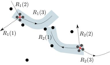
Fig. 3. At the start of each round, we have a set of  $m$  candidate trajectories per robot. The trajectories may be non-uniform and of varying speeds. Using the predicted motion of the targets, we can determine which targets will be covered for a given trajectory and the corresponding quality of tracking.
