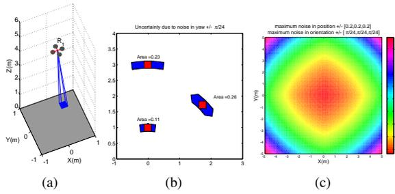
Fig. 1. (a) Backprojection from a pixel yields a pyramid. (b) Uncertainty in target’s estimate due to uncertain yaw angle of the robot. (c) Map showing the area of projection for the true target at  $[x, y, 0]$  (best viewed in color). The camera pose is estimated to have position  $[0, 0, 5]$  m and roll, pitch and yaw angles as 0 radians. Maximum image noise is  $\pm 5$  pixels.
