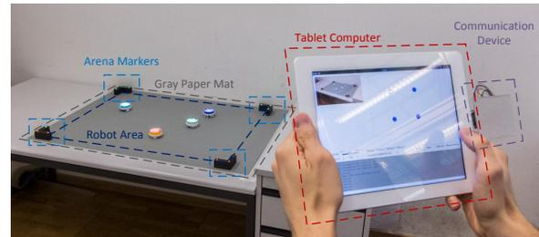
Fig. 1. Several robots and a hand-held tablet for interaction and control.
