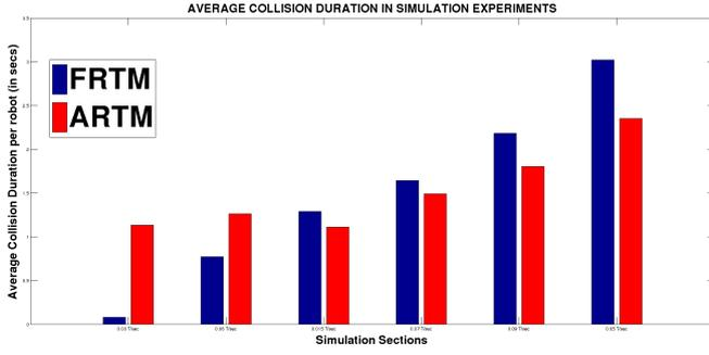
(a) Collision Duration in Simulation Experiments
