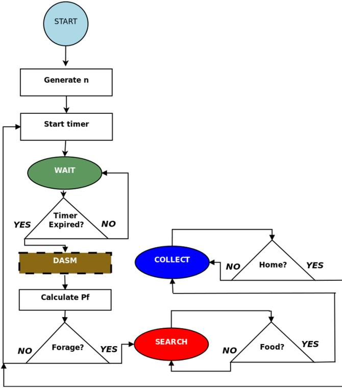
Fig. 2. Task allocation Diagram of ARTM. ARTM's main difference compared to previous methods such as FRTM is the addition of DASM.
